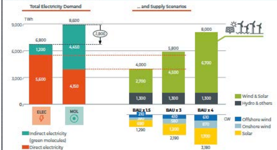
FIGURE 2: STRONG ELECTRIFICATION OF END USE (AS UNDER THE ELEC-PATHWAY) SAVES UP TO 1,800 TWh AT THE EUROPEAN LEVEL COMPARED TO THE MOL-PATHWAY. DIRECT ELECTRICITY DEMAND UNDER THE ELEC-PATHWAY INCREASES BY 70% COMPARED TO TODAY'S DEMAND. A TRIPLING OF TODAY'S RES EXPANSION RATE IS NEEDED TO MEET THIS DIRECT ELECTRICITY DEMAND
